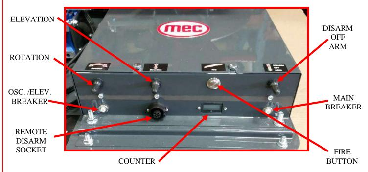
**Rotation Toggle Switch** – Pushing the switch downward will turn the oscillation motor on. Note that the oscillation motor will randomly start/stop when the machine is in operation. This prevents shooters from being able to guess the direction of the next target. Pushing the toggle switch upward allows you to nudge the oscillation motor which pivots the machine from one side to the other enabling you to check the angle of the clays flight.
