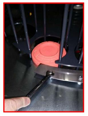
\*\* ALL MEC MACHINES ARE SET UP USING THE WHITE FLYER STANDARD TARGETS. ADJUSTMENTS NEED TO BE MADE WHEN USING OTHER BRANDS OR STYLES OF TARGETS\*\*
