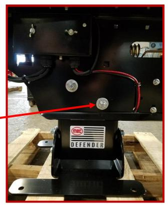
LOOSEN / TIGHTEN THIS NUT TO ADJUST TILT!!
