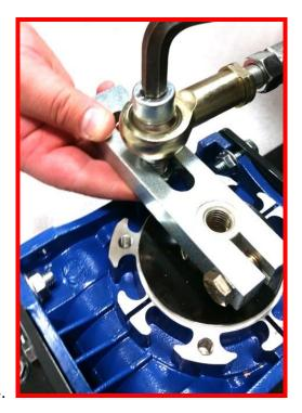
**Step 18** – You can adjust the distance that the clay is thrown by extending the spring. This is achieved by winding tension on or off the main spring using a  $\frac{3}{4}$ " wrench or the optional  $\frac{3}{4}$ " extended socked which can be attached to an impact drive. This should be done with the machine in the disarmed/safe condition for small adjustments.
