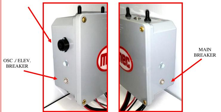
**Rotation Toggle Switch** – Pushing the switch downward will turn the oscillation motor on. Note that the oscillation motor will randomly start/stop when the machine is in operation. This prevents shooters from being able to predict the direction of the next target. Pushing the toggle switch upward allows you to nudge the oscillation motor which pivots the machine from one side to the other enabling you to check the angle of the clays flight.
