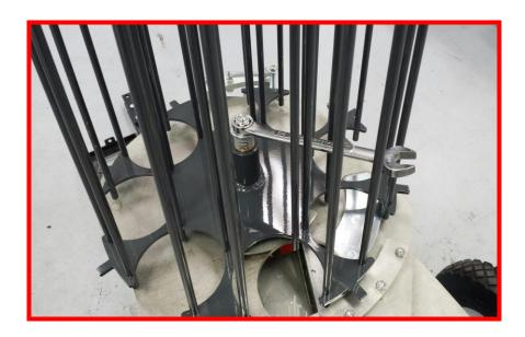
**Step 3** – Check the height / clearance of the knife-edges by placing a clay in the carousel. Rotate the carousel so that the clay starts to pass underneath the inner and outer knife separator blades. The clay must pass freely under the knife separator blades without binding but with the minimum of
