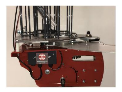
**Step 9** – Adjust the machines tilt by loosening the two black adjustment levers on the base of the machine. There is one at the front and one at the rear of the 300E & 400E machines. Tilt the machine to the desired angle and then retighten both adjustment levers. The angle of the levers can be moved by pulling the lever out and rotating it to the desired position.
