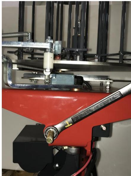
**Step 15** – The pull cord or optional radio release can now be connected to the machine.
