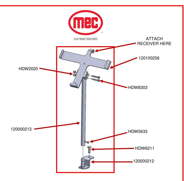
For any questions regarding setup or use of any MEC Clay Target Machines, please give us a call or you can visit us on our website for video footage showing how setup and adjustments are made.
