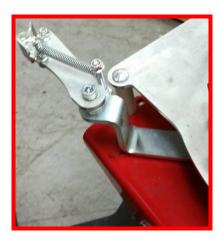
**Step 3** – Swing the plate out towards the front of the machine. This will allow you access the holes in the top plate to attach the shaft. Using the 3 bolts provided simply tighten the shaft to the top plate. For added security Red Loktite can be used, but is not necessary.
