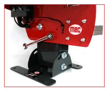
**Step 9** – Adjust the machines tilt by loosening the  $\frac{1}{2}$ "-13 nut on the front and rear on the base of the machine, as shown below. Tilt the machine to the desired angle and then retighten both nuts securely.
