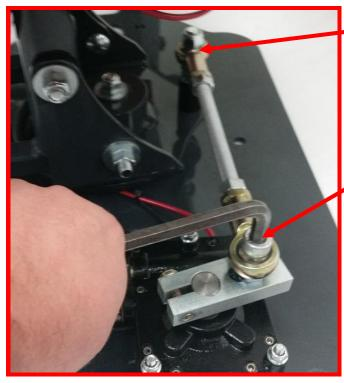
REMOVE THIS END TO ADJUST THE THREADED ROD LENGTH IF NECESSARY!
