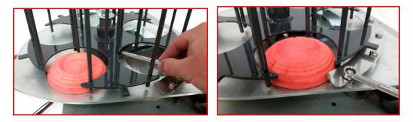
\*\* ALL MEC MACHINES ARE SET UP USING THE WHITE FLYER STANDARD TARGETS. ADJUSTMENTS NEED TO BE MADE WHEN USING OTHER BRANDS OR STYLES OF TARGETS\*\*
