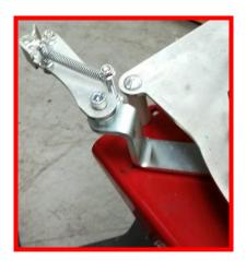
**Step 3** – Swing the plate out towards the front of the machine. This will allow you access the holes in the top plate to attach the shaft. Using the 3 bolts provided simply tighten the shaft to the top plate. For added security Red Loktite can be used, but is not necessary.
