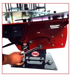
**Step 9** – Adjust the machines tilt by loosening the  $\frac{1}{2}$ "-13 nut on the front and rear on the base of the machine, as shown below. Tilt the machine to the desired angle and then retighten both nuts securely.
