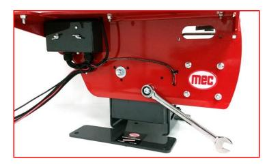
**Step 9** – Adjust the machines tilt by loosening the  $\frac{1}{2}$ -13 nut on the front and rear on the base of the machine, as shown below. Tilt the machine to the desired angle and then retighten both nuts securely.
