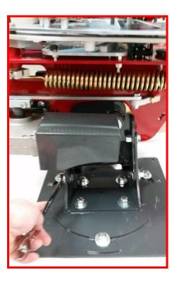
**Step 10 –** Rotate the machine by loosening the three 1/2" nuts. Once the machine is rotated to desired position, retighten the three nuts to secure machine.
