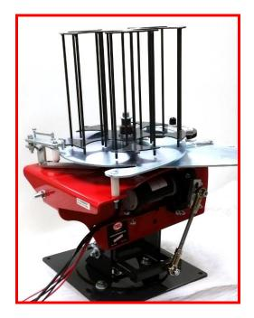
**Step 9** – Adjust the machines tilt by loosening the  $\frac{1}{2}$ -13 nut on the front and rear on the base of the machine, as shown below. Tilt the machine to the desired angle and then retighten both nuts securely.
